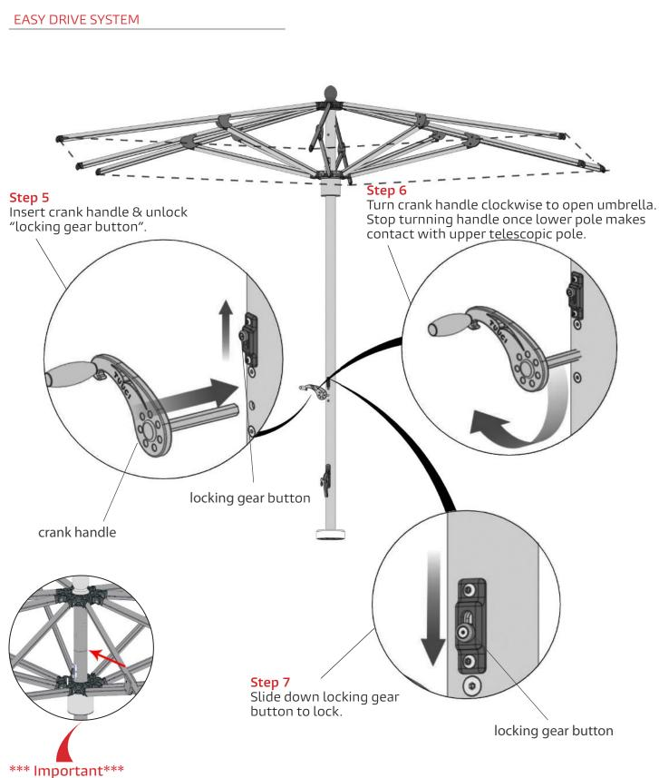
Do not overcrank. Stop when top telescopic head makes contact with main umbrella pole
