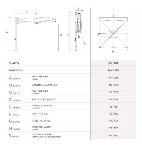
Dimension Tolerances  $\pm 2^{\prime\prime}/5$ cm. Dimensions shown are rounded to the nearest inch and correspond to indicated lift system. Options are subject to change without notice.
