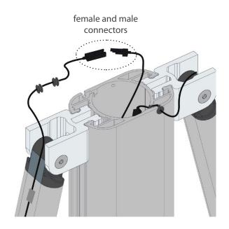
Step 8 Insert 1st grommet on inner mast groove by runing cables through clips
