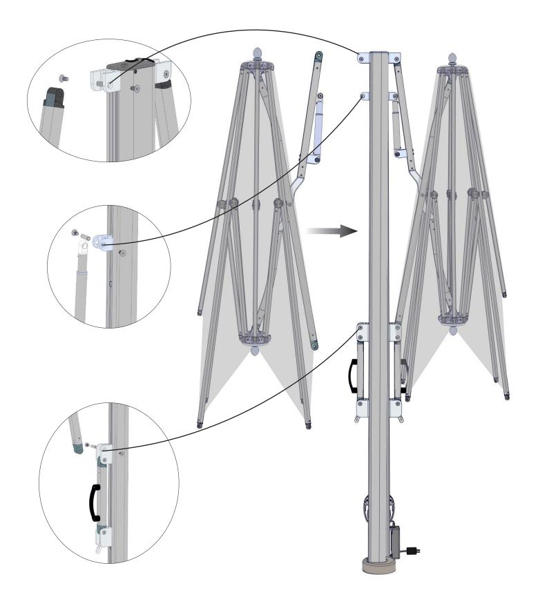
**Step 6** Remove cap screw and mast cap and clip.
