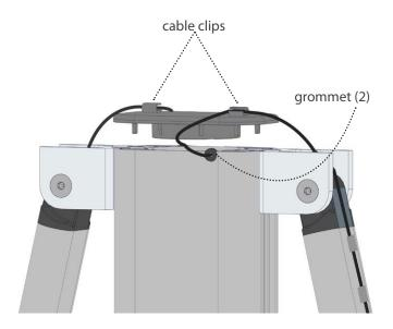
Step 10 re-install cap and screws
