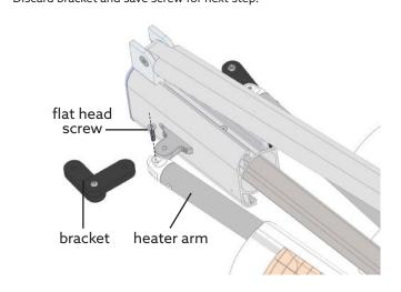
**Step 4**Mount heater arm to elbow fitting with flat head screw
