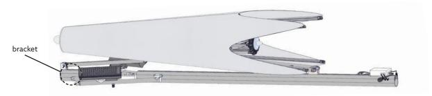
**Step 2**Remove hex screw from elbow fitting.
