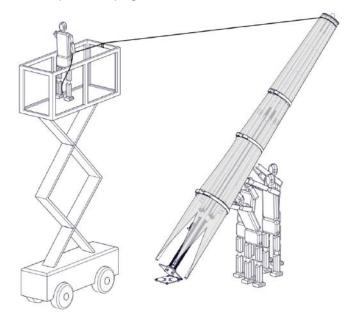
**Step 11**Use the provided hardware to secure the hinge base.
