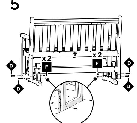
Note: Installing the base backwards could result in unexpectedly tipping over.
