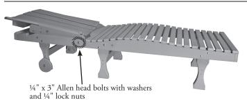
STEP #2 - Fasten the back to the seat using ¼" x 3" Allen head bolts with washers and ¼"lock nuts. (See motion point diagram A.)
