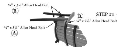
**A.** Attach the seat to the back using 1-  $\frac{1}{4}$ " x  $3\frac{1}{4}$ " Allen Head Bolt and Flange Nuts.
