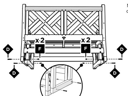
Note: Installing the base backwards could result in unexpectedly tipping over.
