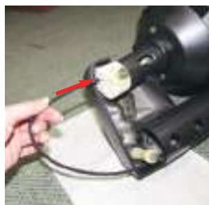
Pull cord out and over to insert cord through top left side of white cap. Continue to feed cord through until cord is fully inserted.
