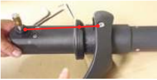
Make sure crank shaft is lined up with tilt lever bolt.
