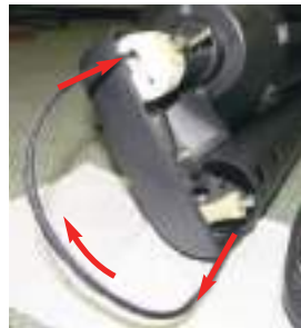
Pull cord out and over to insert cord through top left side of white cap. Continue to feed cord through until cord is fully inserted.
