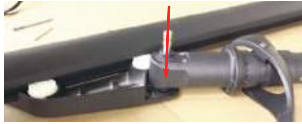
Set crank handle mechanism into grip handle housing.
