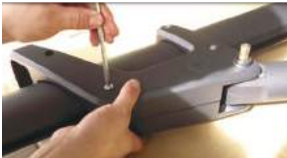
Attach nut under grip housing and tighten each of the 4 bolts to each nut using a 6mm hex wrench.
