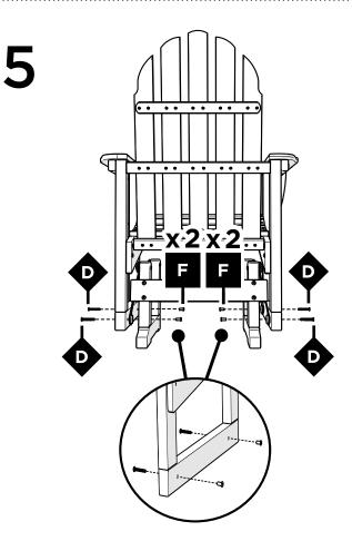
Note: Installing the base backwards could result in the glider tipping over unexpectedly.
