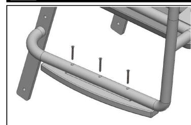
On a clean flat surface align armrest with slot and attach using (3) 1 5/8" Phillips head screws. Repeat on opposite side. Do not over tighten.
