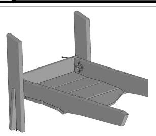
Attach front apron of Seat Assembly to Front Legs with (2) 1-3/4" Phillips Head Screws as shown using a #2 Phillips head screwdriver.
