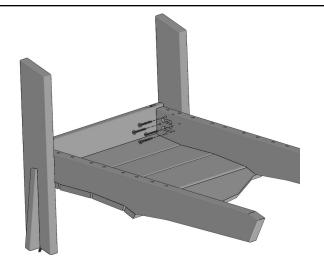
Align Front Leg Assemblies with Seat Assembly. Secure using (8) 50 mm Connecter Bolts thru threaded inserts in Legs using a 4mm Allen wrench.
