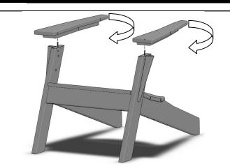
Align threaded insert in front of Arm Assemblies with hanger bolt in front legs. Spin clockwise until aligned and tight. A A Sh
